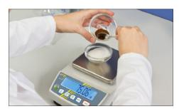
With the **recipe function** you can weigh the different ingredients of a mixture. For control purposes you can also call up the total weight of all the ingredients
